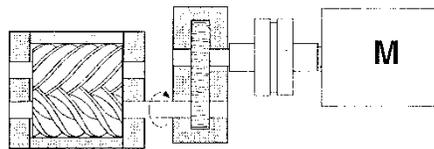
Because of reduced volumetric efficiencies at low speeds, most small screw compressors are fitted with gears or pulleys to increase the rotor speed
